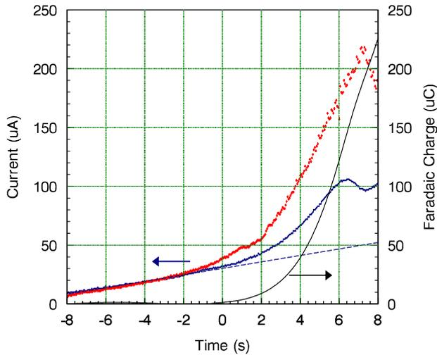
Fig. 9. Current conducted through an electrode pair in still PBS subjected to a ramp voltage stimulus (solid joined dots) is plotted along with the same in agitated solution (scattered symbols). Also shown is the linear extrapolation of the portion before the diodes turn on (dashed line). Finally the net Faradaic charge conducted through the diode-memristor combination (solid line).
