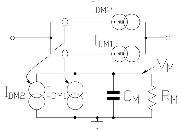
Fig. 6. The subcircuit used to implement the diode-memristor branches.  $I_{DM1}$  and  $I_{DM2}$  represent the two terms of equation (14), evaluated using (16) and (17). Charge conducted through the two diode-memristor branches is accumulated in capacitor  $C_M$ , giving rise to voltage  $V_M$  that is subsequently used to calculate  $I_{DM1}$  and  $I_{DM2}$ .
