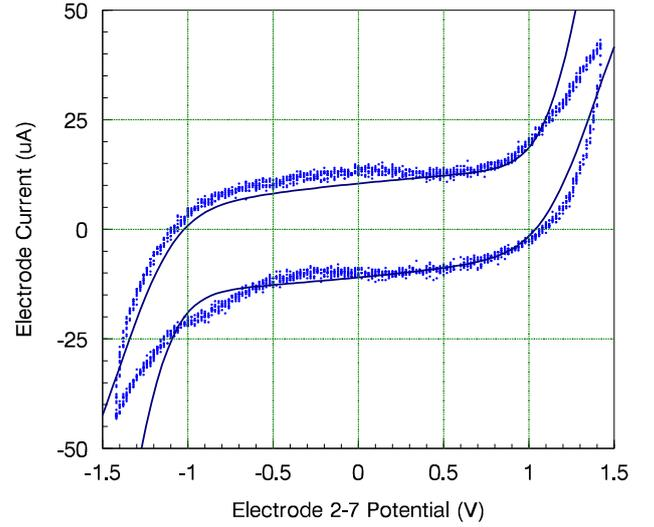
Fig. 8. Voltage across versus current through an electrode pair stimulated with a medium-signal, 20mHz, triangle wave. Symbols are measured data, the continuous line is simulated data.
