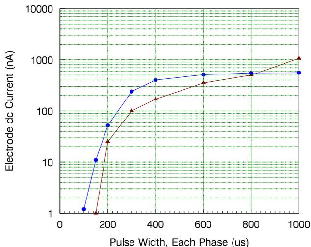
Fig. 12. Measured (triangles) and simulated dc current that flows when a 6mA biphasic pair of pulses with  $50\mu\text{s}$  spacing and varying width are applied between electrodes 2 and 7 on an Octrode.
