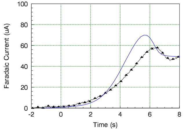
Fig. 10. An estimate of measured Faradaic current conducted through an electrode pair in still PBS subjected to a ramp voltage stimulus, along with the simulated value. Measured data is marked with triangle symbols.
