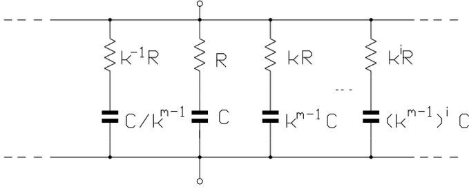
Fig. 4. Infinite-RC-series model of a constant-phase element, after [14]. The counter  $i$  ranges such that the time constant  $\tau$  of the first and last branch span the required bandwidth. The parameter  $k$  is chosen to set the “density” of branches which is related to the accuracy of the approximation.
