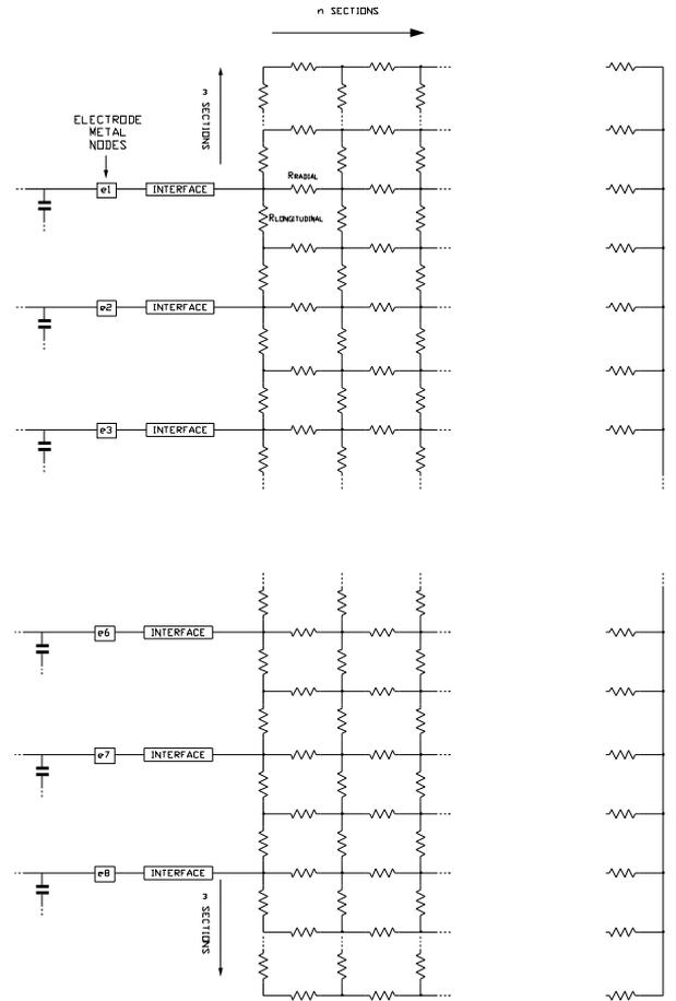
Fig. 2. Schematic of the model of the 8-electrode array in electrolyte. The interface properties are modelled by the branches marked “interface”.
