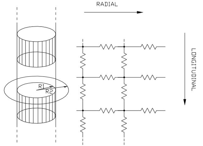
Fig. 1. Geometry of a section of the cylindrical electrode array showing two electrodes (shaded) and an insulating segment with a snippet of the resistor mesh to be derived from the conducting electrolyte that surrounds the electrode array.
