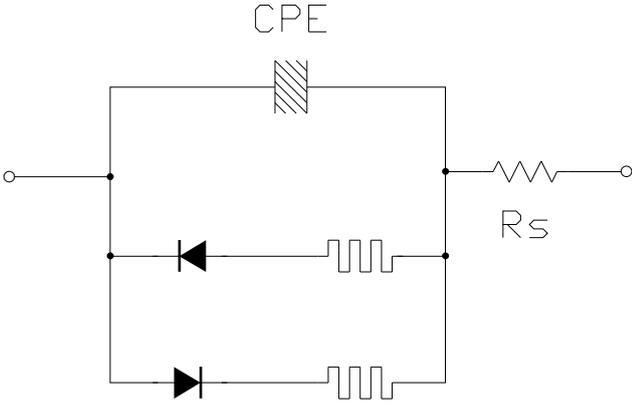
Fig. 5. Proposed model of the electrode-electrolyte interface, containing a constant-phase element, two diodes, two memristors, and a series resistance.
