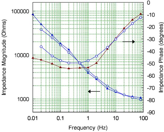
Fig. 7. Magnitude and phase versus frequency of the small-signal impedance from stimulated electrode to an adjacent electrode, representing electrode impedance plus a small contribution from the resistor grid. Measured data is marked with triangles, simulated data with circles.
